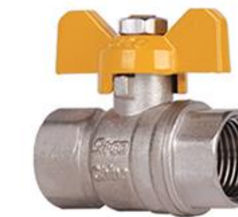
Ball Valve With Butterfly Handle Size: 1/2" & 3/4" Material: Nickel Plated Brass Body Chrome Plated Brass Ball
