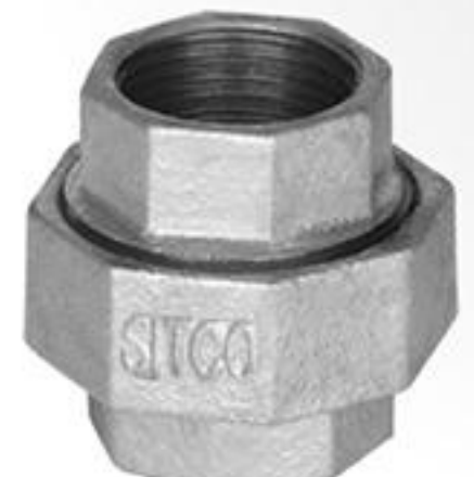
Threaded Union Material: Hot Dipped Galvanized Pressure Resistance: 2 to 2.5 Mpa
