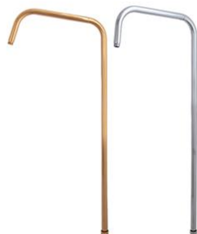
SS Shower Pipe Material: SS 201 / SS 304 Length: 1280 mm Diameter: 22 mm Thickness: 0.5 mm Finish Chrome / Gold
