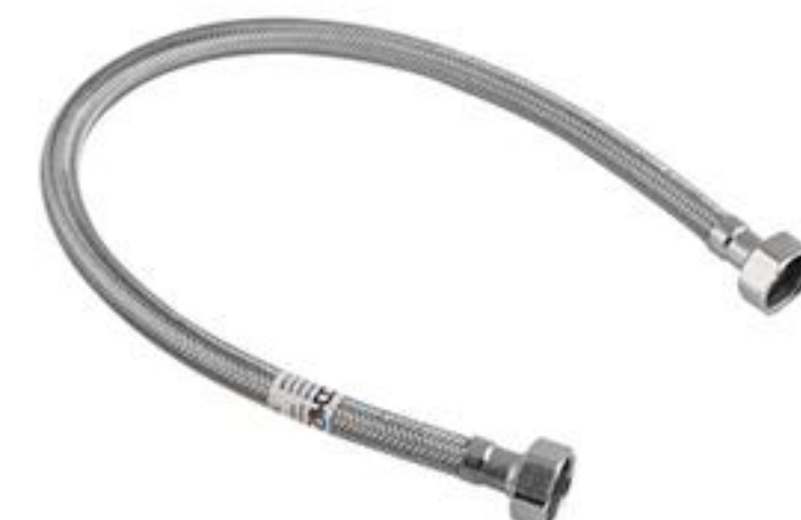
Two Headed Hose Length: 30 & 40 & 50 & 60 & 70 CM Dia: 12 MM / Size: 1/2" Material: SS - EPDM - Brass
